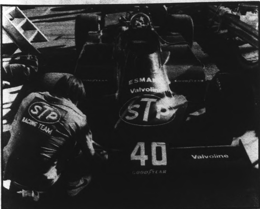
Owen Syneder of the Patrick Racing Team places tape on the front wing of Mario Andretti's Wildcat Cosworth in order to cut down on aerodynamic drag. Rough edges on the car can reduce handling and top speed.
