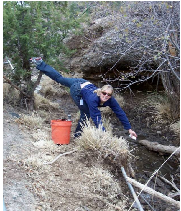
Figure 6 – ADEQ's Elizabeth Boettcher collects a sample (UHA-31) from Collins Spring located in the Prescott National Forest. Analytical results indicated the Secondary MCL for manganese was exceeded.
