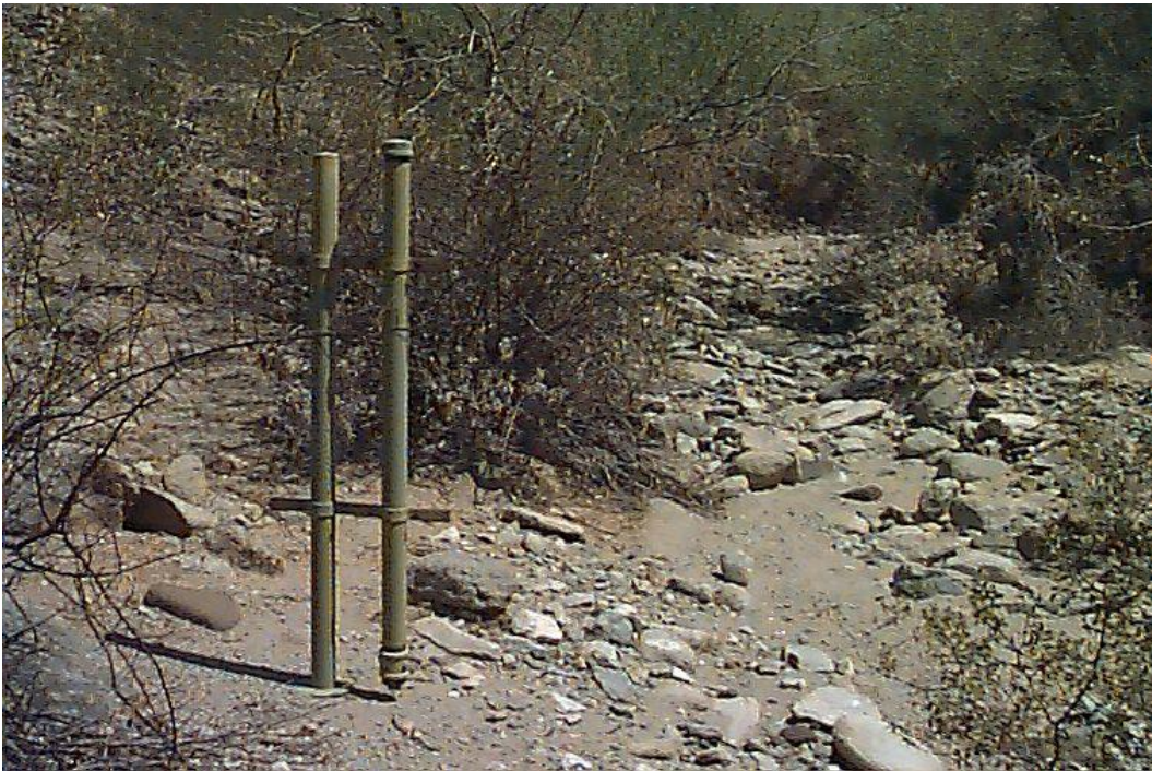
Figure 6. Photograph of a crest gage, located upstream of the weather station at Sierra Estrella Fan.
