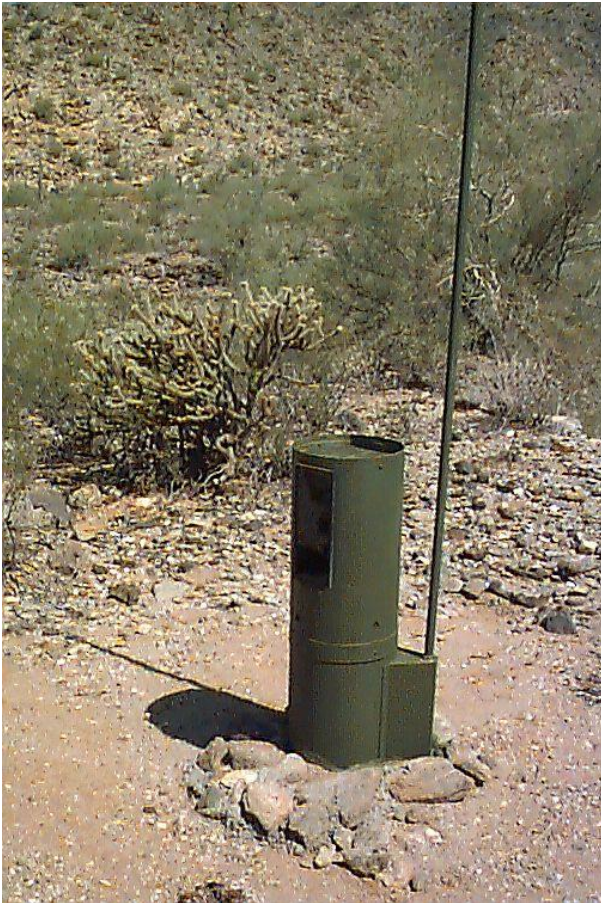
Figure 7. Photograph of tipping bucket number 6870, located in the upper watershed of Sierra Estrella Fan.
