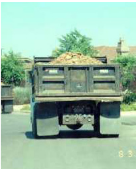
Load height violation
