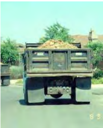
Load height violation
