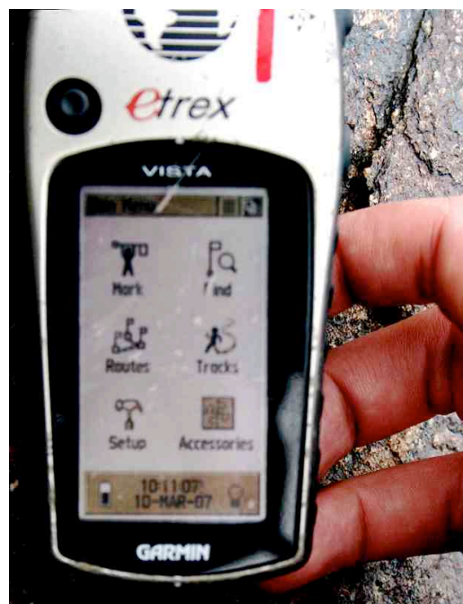
Figure 4: GPS clock is at the bottom of this screen on the Garmin eTrex™.
