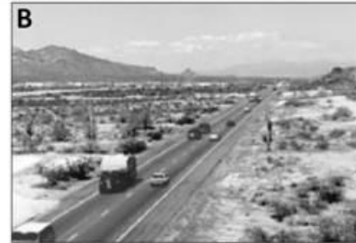
LOS B: Traffic is slightly more congested, with some constraints on maneuverability. Two motorists might be forced to drive side-by-side, limiting lane changes; however, traffic speeds are not reduced.
