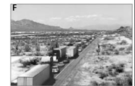
LOS F: Facilities operating at LOS F generally have more demand than capacity. LOS F is the lowest measurement of efficiency for a road's performance. Traffic flows will be below the posted speed and experiences reduced travel times due to heavy congestion.
