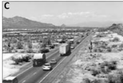
LOS C: Congestion is greater than LOS B, where ability to pass or change lanes is not always assured but the posted speed is maintained. Most experienced drivers are comfortable, and roads remain safely below but efficiently close to capacity.
