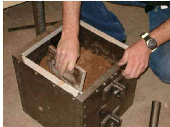
(b) Compacting material layer
