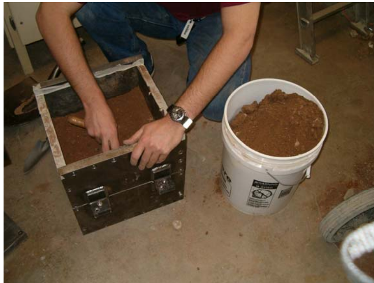
Figure 77: Material is removed from the upper half of the box.
