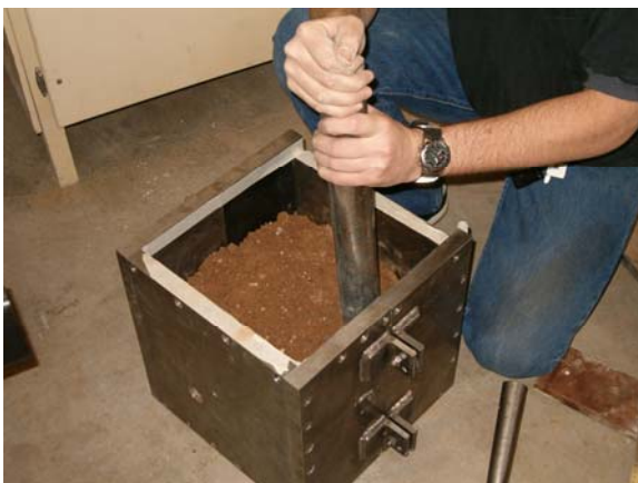
(c) Compacting material layer
