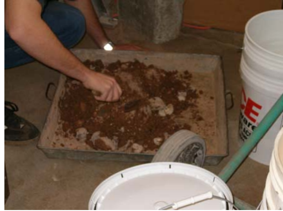
(b) Water is added and mixed wet
