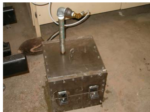
(f) Applying Air Pressure to Concrete
