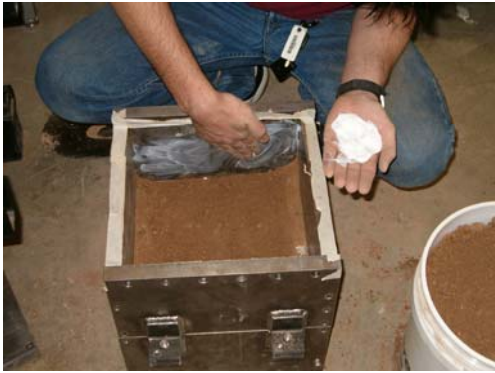
(a) Box Upper Half is Coated with Vaseline
