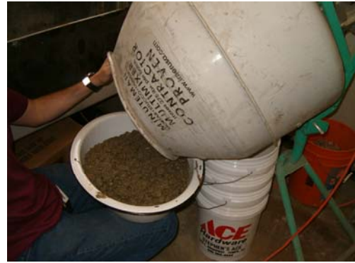
(b) Concrete Poured from Mixer
