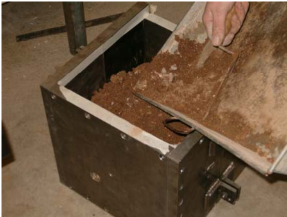
(a) Material is poured into the box
