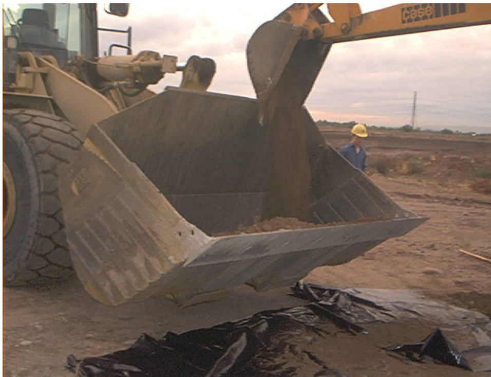
Figure 48: The Material is Dumped (collected) in a Loader to be Weighed.
