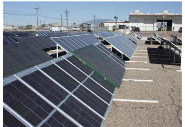
AzRISE / Tucson Electric Power (TEP) Solar Test Yard, an interdisciplinary research project to acquire and distribute data in the measurement of solar panel performance, PV production models and studies in techniques that increase the energy yield from PV systems.
