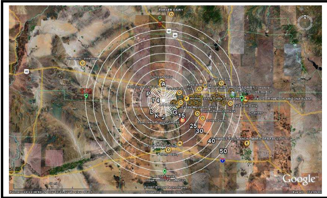
AN AERIAL VIEW OF THE 50 MILE PALO VERDE PLANNING ZONE, ESTABLISHED IN CASE OF WIND DRIFT OF RADIOACTIVE MATERIALS AWAY FROM THE PLANT. THE 10 MILE EMERGENCY ZONE WOULD BE A PRIMARY FOCUS DURING AN EMERGENCY.
