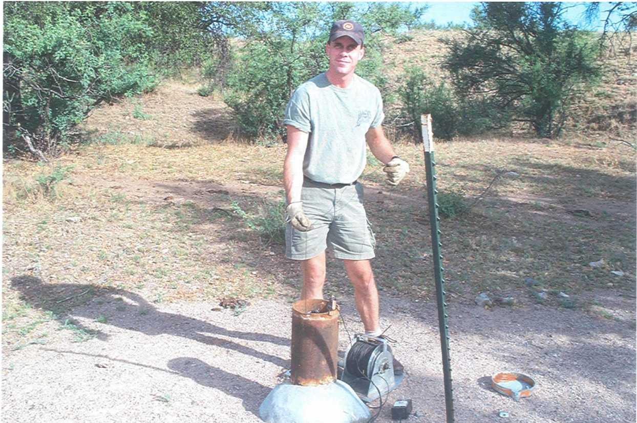
Figure 2. Department personnel measuring groundwater levels in a well drilled into the older alluvium south of Potrero wellfield (G12).
