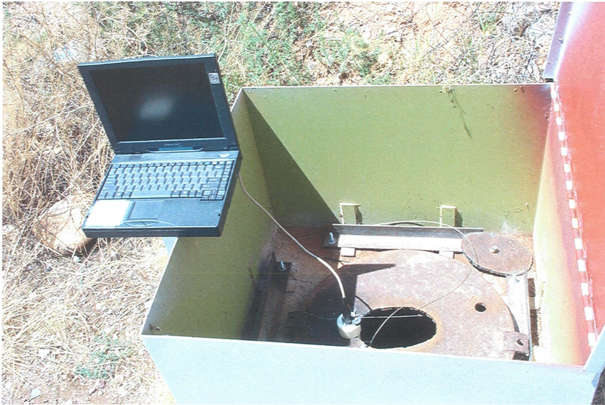
Figure 9. Downloading data from pressure transducer at a well near Elephant Head Bridge (G1).
