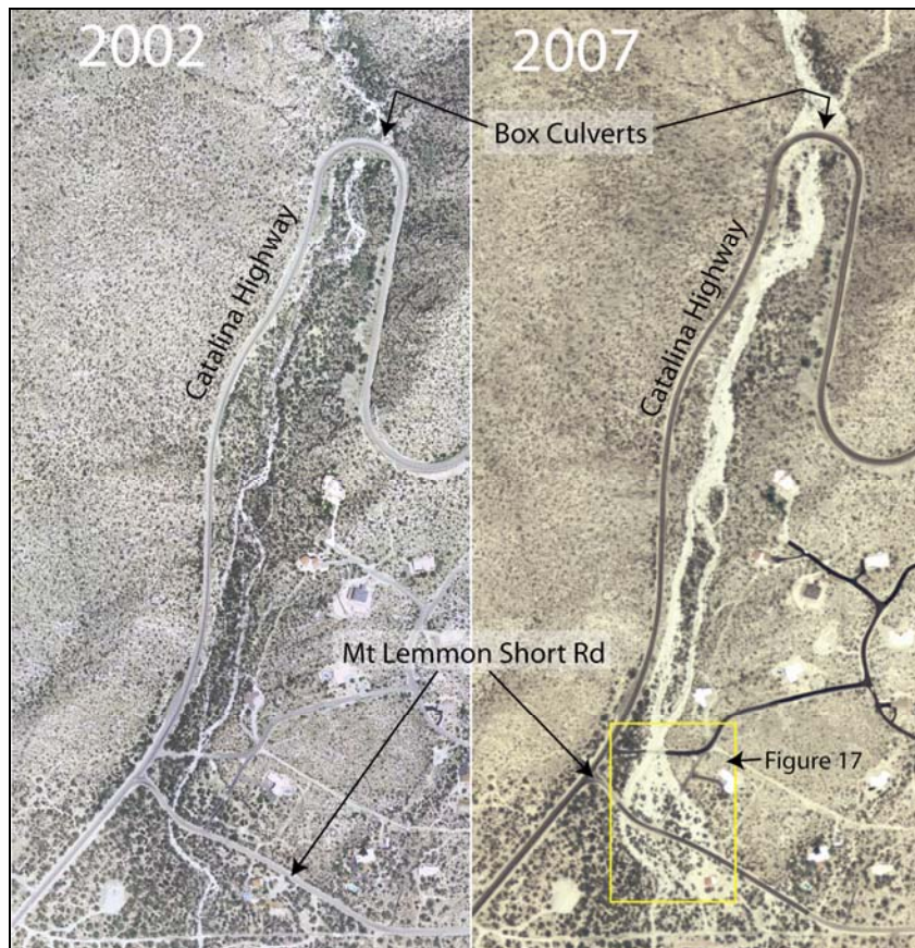
Figure 16. Comparison of Soldier Wash channel between 2002 (left) and 2007 (right). Debris flows and floods significantly widened the channel; older, abandoned channels were re-occupied. Yellow box shows area in Figure 17.
