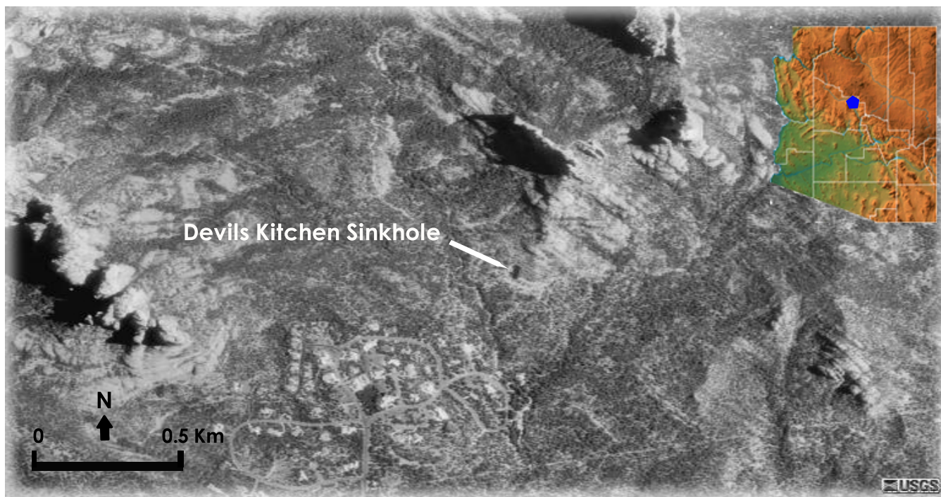
Figure 1. Aerial photograph showing Devils Kitchen Sinkhole situated north of Sedona, Arizona. Note the pervasive north west trending joint system. Inset map shows the approximate location of the study area.
