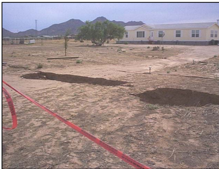
Fig. 17 – Earth fissure gully that reopened August 2005 near residences south of Queen Creek, Arizona – led to the enactment of HB2639 (photo by Mike Schaffer)
