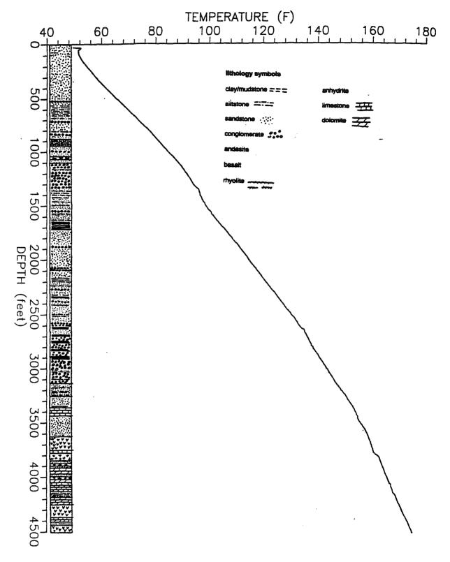
Figure 6. Equilibrium temperature versus depth for the Alpine 1/Federal borehole.
