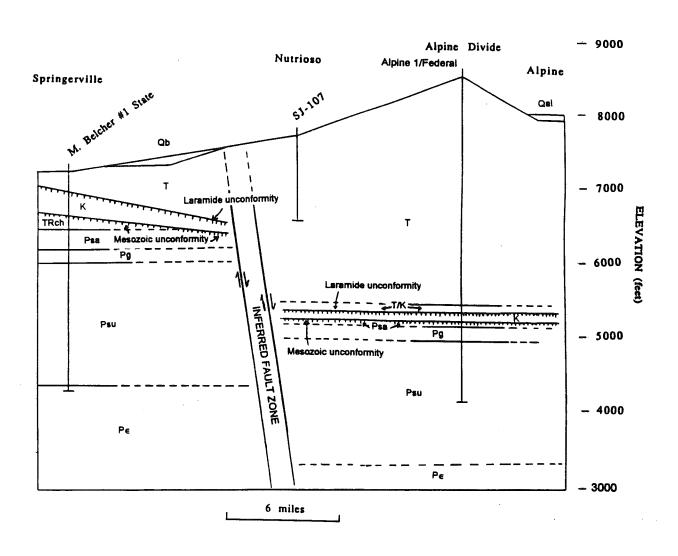
Figure 5. Post-drilling geologic model of subsurface geology.
