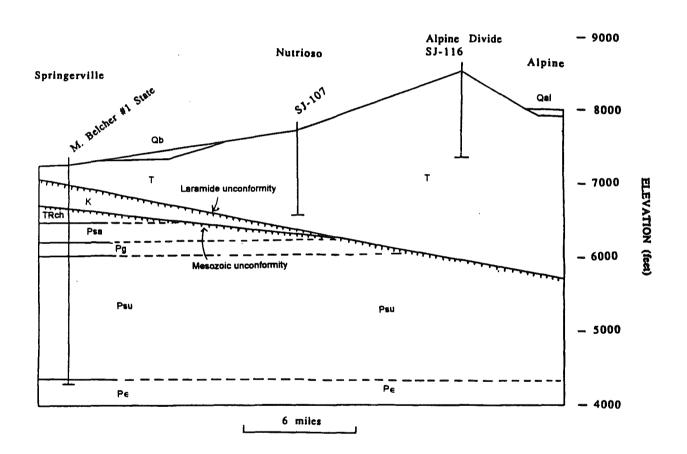
Figure 4. Pre-drilling geologic model of subsurface geology.
