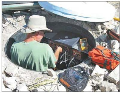
**Figure 4:** Bigfoot seismometers are housed in a well in order to dampen out seismic noise. Photo courtesy of EarthScope.
