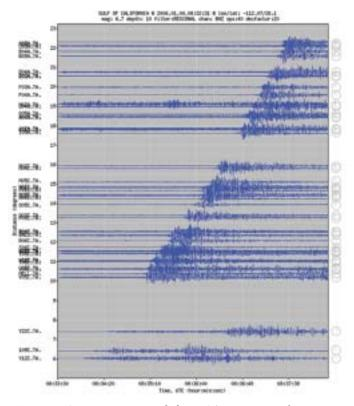
**Figure 5:** Seismograms recorded at USArray stations from a magnitude 6.7 quake that occured in the Gulf of California on January 4, 2006. Courtesy of the IRIS DMC WILBER II system and Matt Fouch, Arizona State University.
