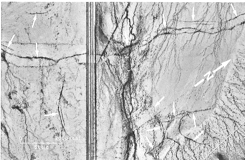
Figure 3. Aerial view of same area shown in Figure 2, taken 14 years later. Proliferation of earth fissures is indicated by arrows. Note that subsequent fissuring near the original fissure is all on the basin (west) side. Other fissuring, which may be due to buried bedrock topography, is evident to the east. Photo taken on January 9, 1978 by the Arizona Department of Transportation.
