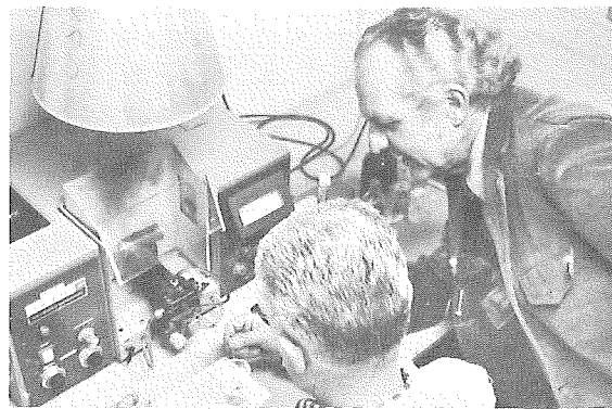
Small particles are sometimes quantitatively assayed by ATOMIC ABSORPTION SPECTROGRAPHIC ANALYSIS to gain knowledge of a mineral's chemical formula.
