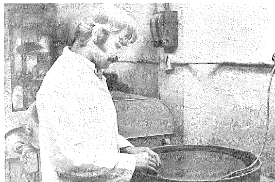
Bureau laboratory assistant Tom McGarvin prepares a THIN SECTION—a slice of rock 3/1000" thick, mounted on a slide. Microscopic examination will reveal the optical properties of the minerals in the rock.
