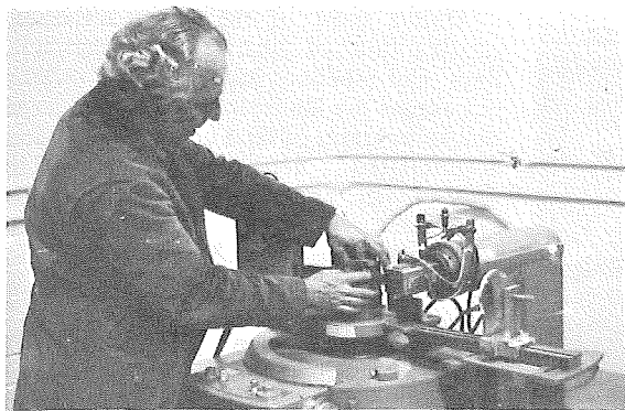
By X-RAY DIFFRACTION ANALYSIS, the mineralogist can establish a mineral's crystal lattice structure—the patterns that atoms assume in a mineral—thereby aiding mineral identification. In general, all minerals have unique crystalline structures by which they can be distinguished, even when composed of the same elements.
