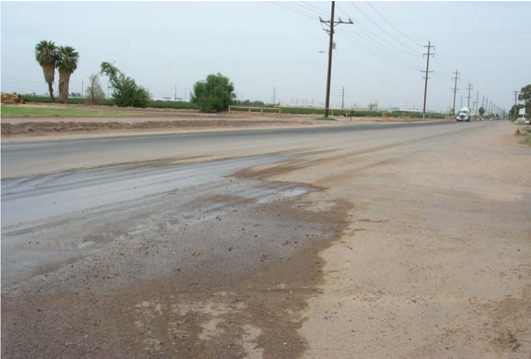
Figure D-3. Sample #3 (above photo) taken on the northbound lane of 43 rd Avenue, 910 feet north of origin (area dimensions = 2 feet by 18 feet). Sample #4 taken directly across (west) from Sample #3 on the southbound lane, just north of exit road from the dirt storage pile (area dimensions = 6 feet by 18 feet). Photo is looking northwest.
