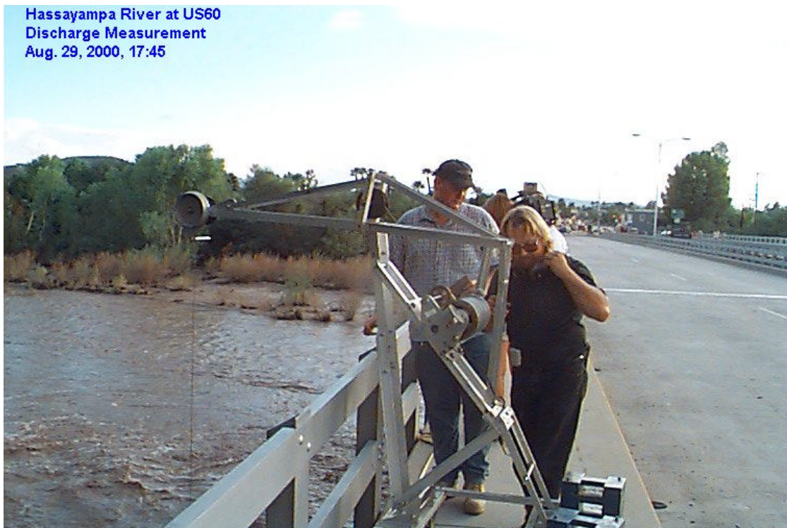
FCD crew taking a flow measurement on the US 60 Bridge over the Hassayampa River
