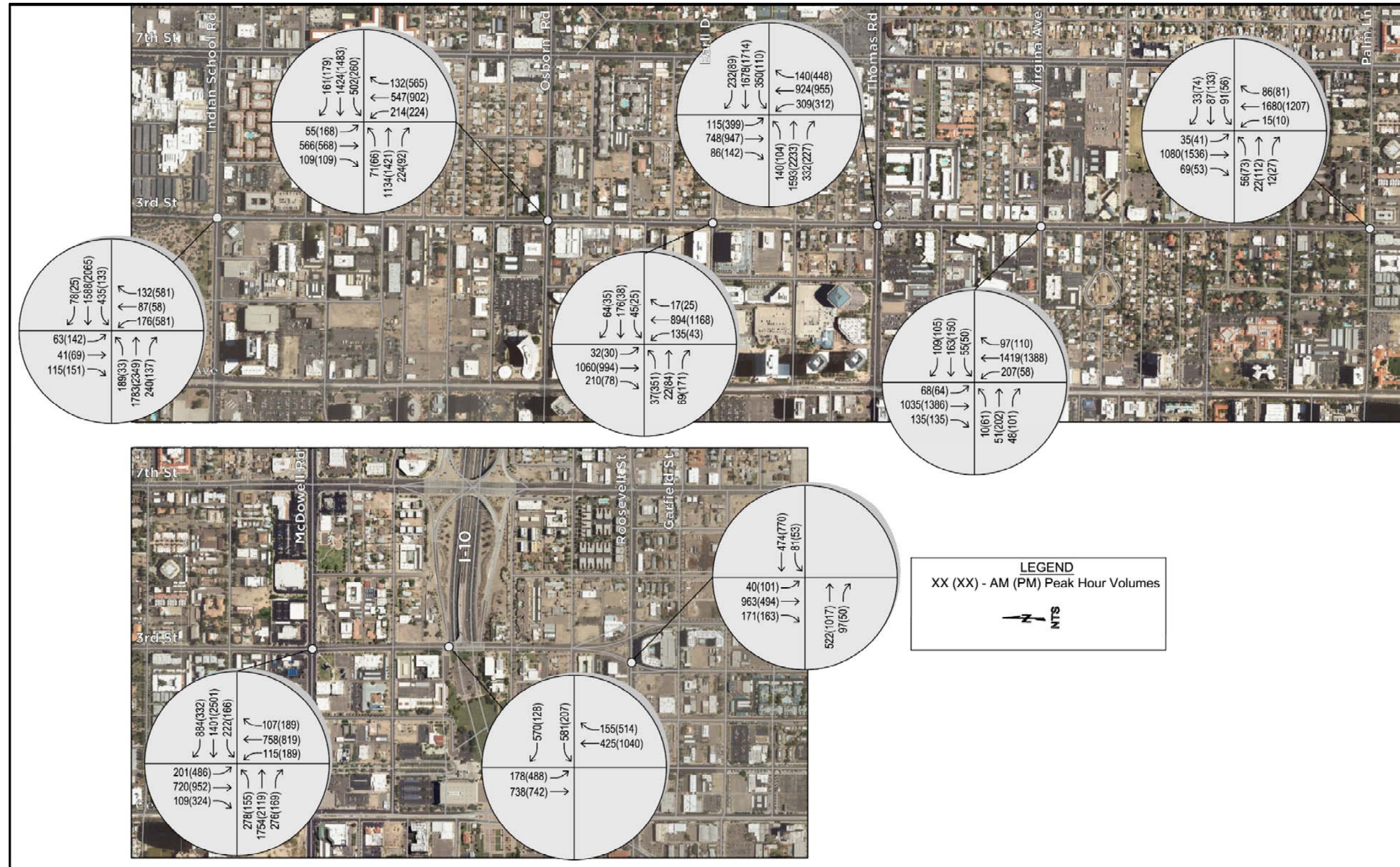
Figure 20 - Third Street Corridor 2035 Intersection Turning Movement Volumes
