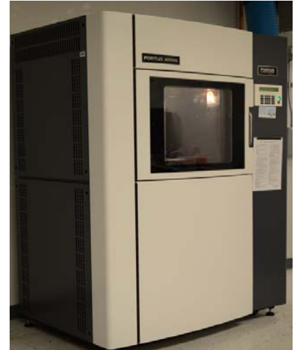
Stratasys Fortus 400MC 3D Printer, which has the ability to create prototypes and production-grade parts using high-performance thermoplastics.
