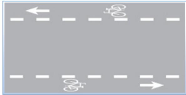
Typical Striping for Bike Lane on Roadway
