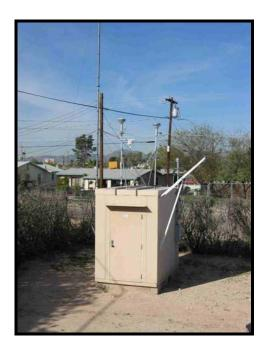
**Comments:** This monitor was initially installed in July 1, 2007 for Air Quality Index reporting using a continuous monitor. This is a Special Purpose site situated in a residential area, monitoring for population exposure.
