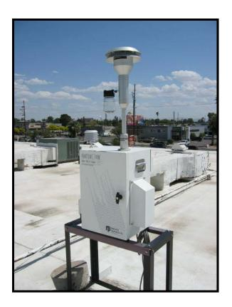
**Comments:** In August of 1990 this site was relocated from an adjacent building. In May 2006, the colocated sampler was retired and the Hi-Vol sampler was replaced with a Low-Vol R&P 2000 sampler. The site was closed October 31, 2010 because roof space was no longer available.
