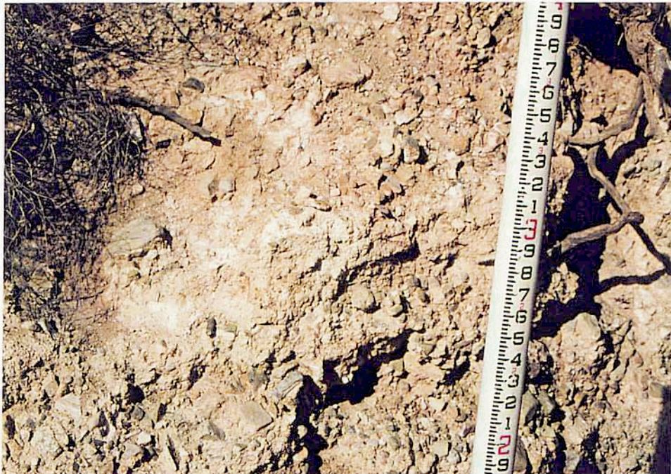
Photograph 10 - Close up of west bank located slightly downstream of photo 9, behind Lots 226 & 227. Notice calcification (white) of bank material.
