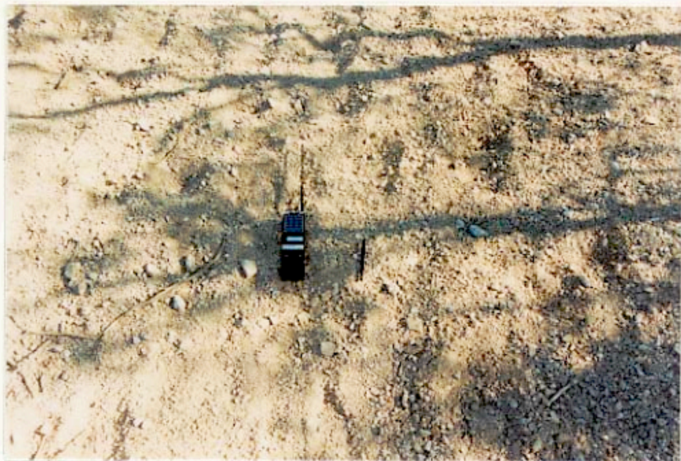
Figure 3 Composition of the wash bed is made up of small angular rock which would reduce the potential for the channel to deepen.
