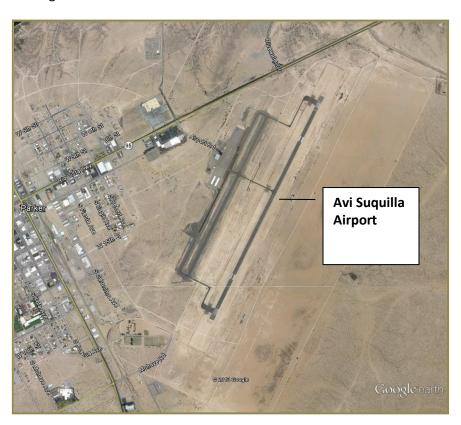
Airside facilities consist of runways, taxiways, and apron areas along with associated markings, lighting systems, and instrumentation. The existing runway configuration consists of one active runway, Runway 1-19. It is 6,250 feet long and 100 feet wide. There are also two taxiways aligned with Runway 1-19 and several connecting taxiways.
