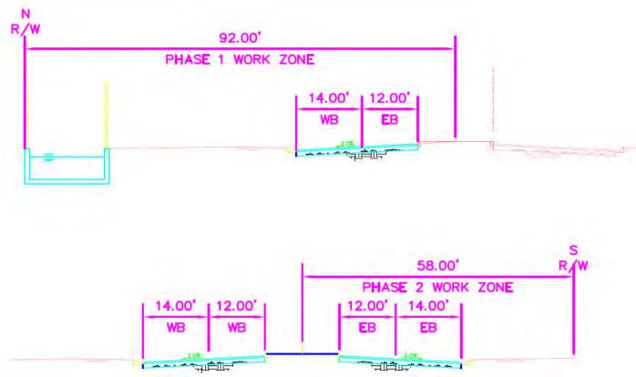
Figure 5- Phased Construction of Grace Neal Parkway. (Looking East. NTS)
