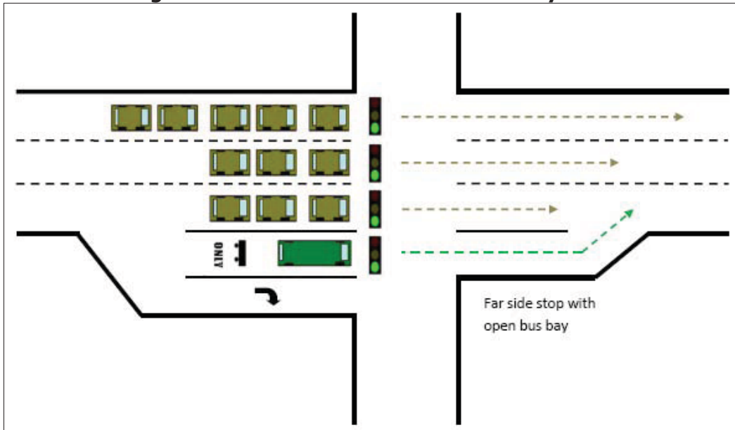
Figure 20: Intersection with Bus Priority Lane
