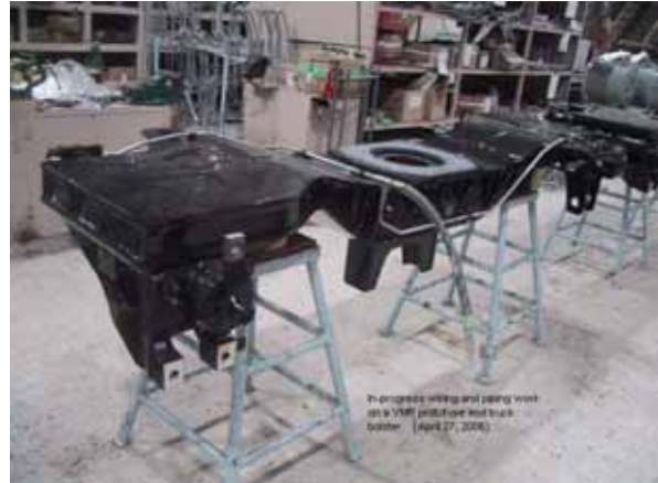
In progress wiring and piping work on METRO prototype end truck bolster April 27.
