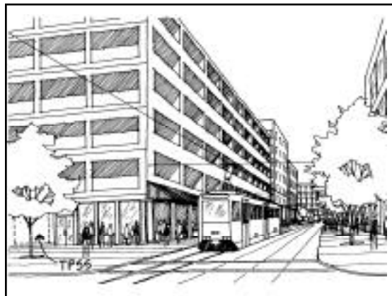
TPSS in Nearby Structure
