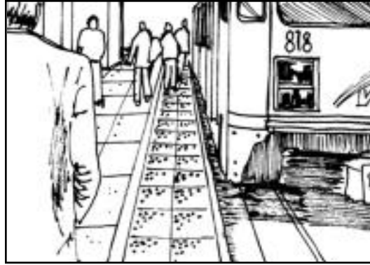
Tactile Strip on Side Platform
