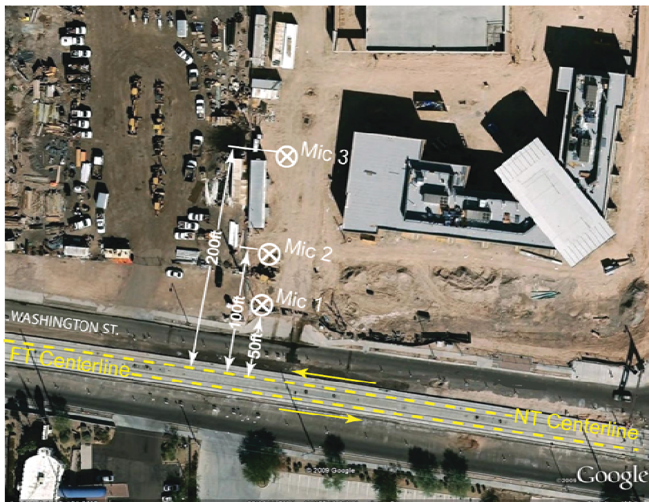
FIGURE D-1: AERIAL VIEW OF MICROPHONE LOCATIONS FOR LRT NOISE MEASUREMENTS
