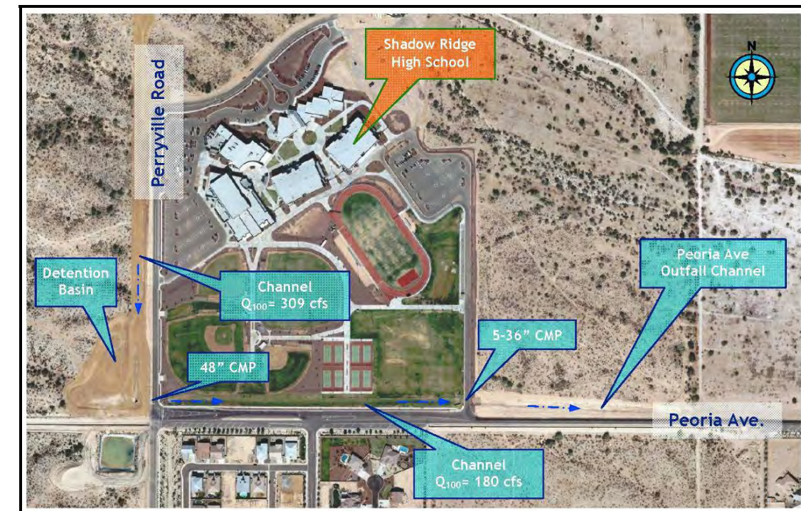
Figure 8 - Shadow Ridge High School Off-site Drainage Facilities
