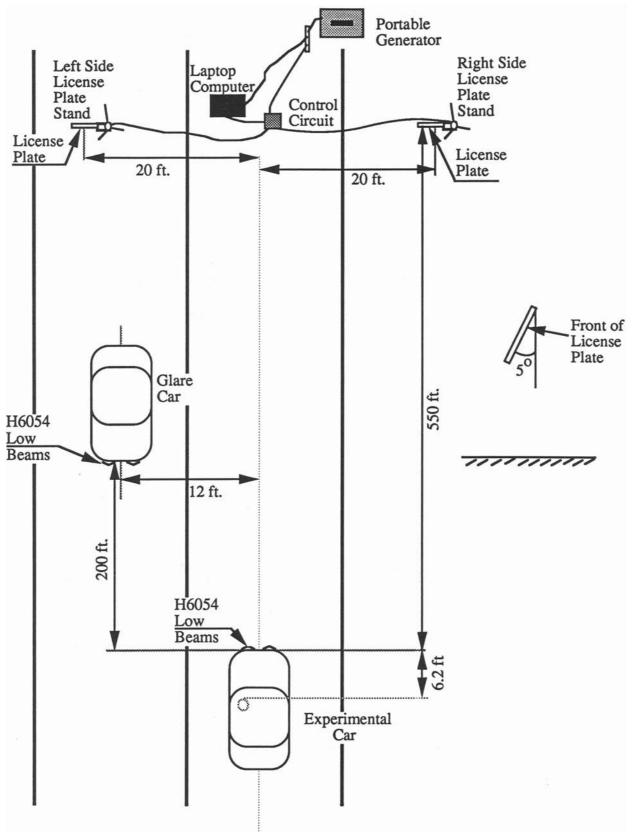
Figure 2. Setup for Nighttime Conspicuity Experiment
