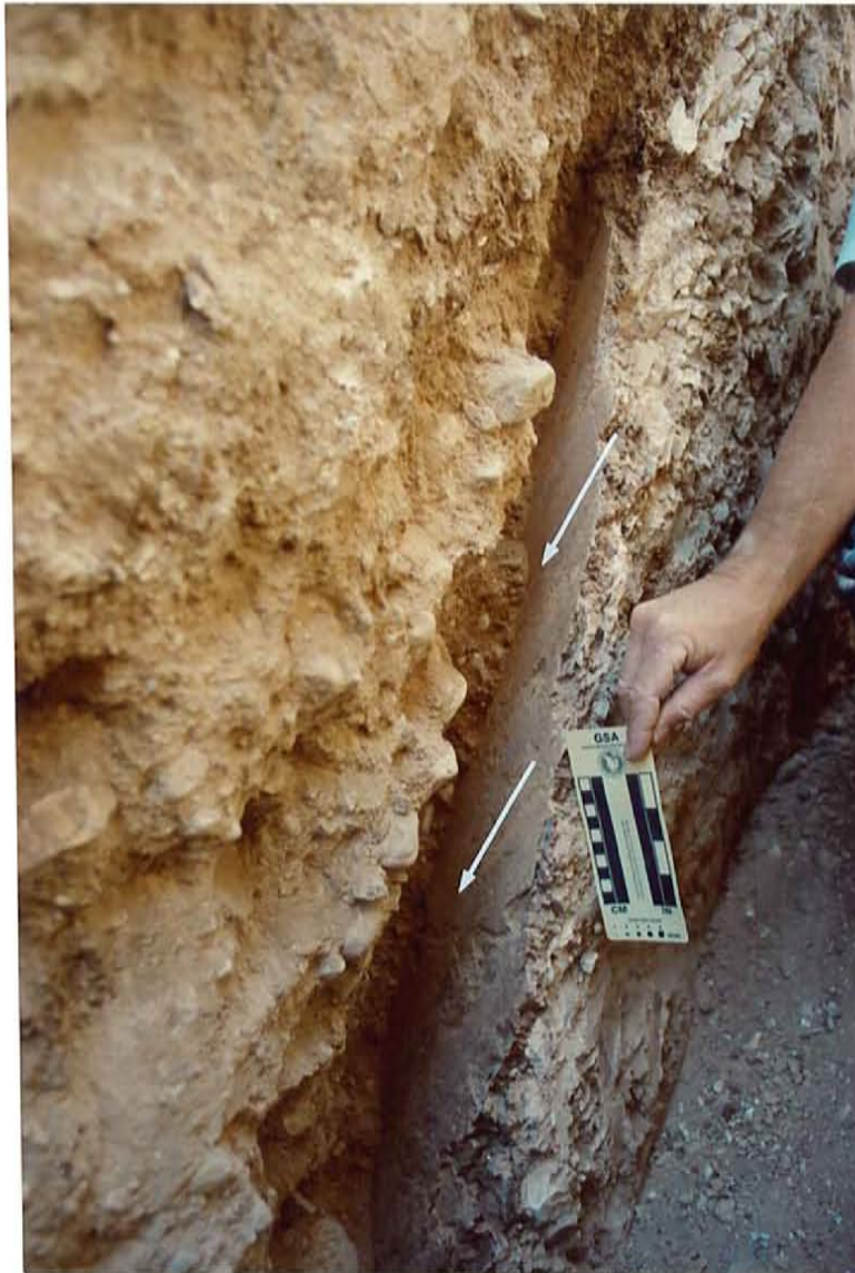
BETWEEN STATIONS 50-55 ON TRENCH LOG, TRENCH NO. 3. NOTE GROOVES AND STRIATIONS (SLICKENSIDES) ON SMOOTH POLISHED FAULT-PLANE SURFACE. ARROWS SHOW 60 DEGREE, OBLIQUE ORIENTATION OF SLICKENSIDES. GSA CARD SHOWS SCALE IN INCHES AND CENTIMETERS.
