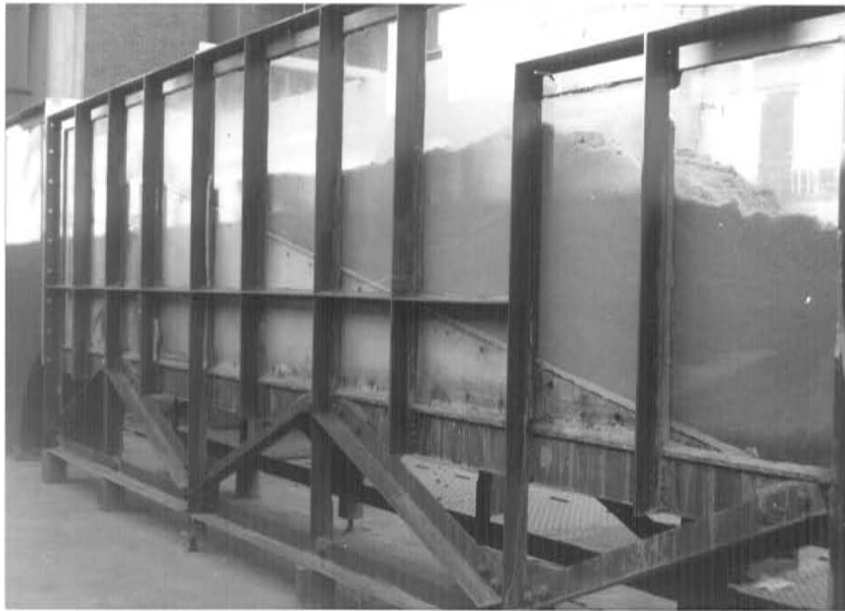
FIGURE 10. Flume for Scour Study.
