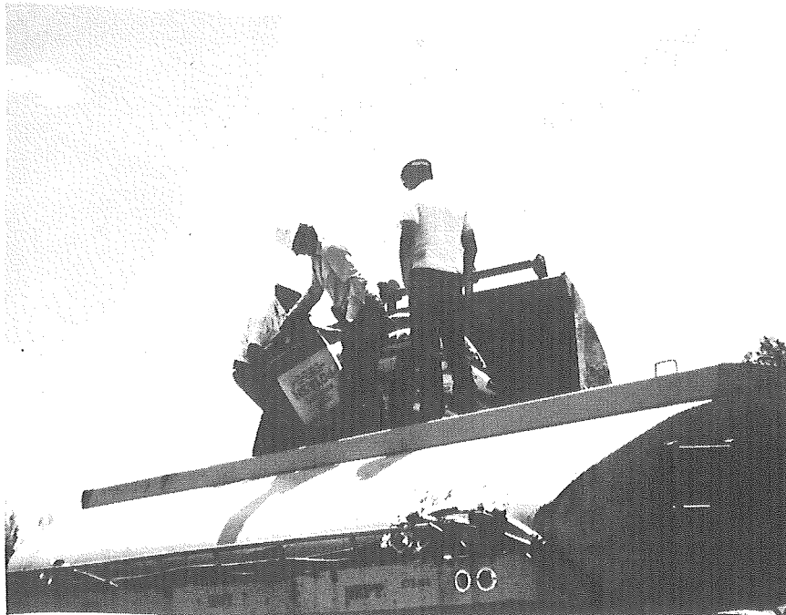
Figure 33 shows one of the sixty 100 pound (45.4 KG) KCL bags being emptied into the water filled tanker.
