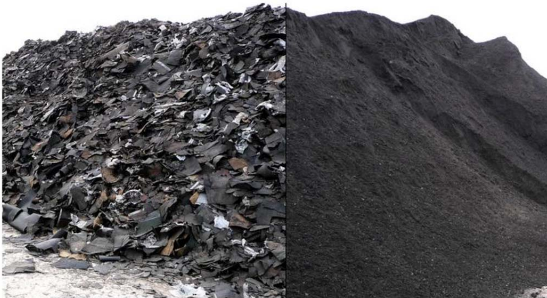
Figure 6. Unprocessed Post-Consumer Shingles (Left) and Processed RAS (Right) (ARSR 2012)
