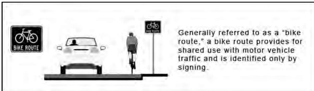
Figure 16: Typical Bike Route Cross-section
